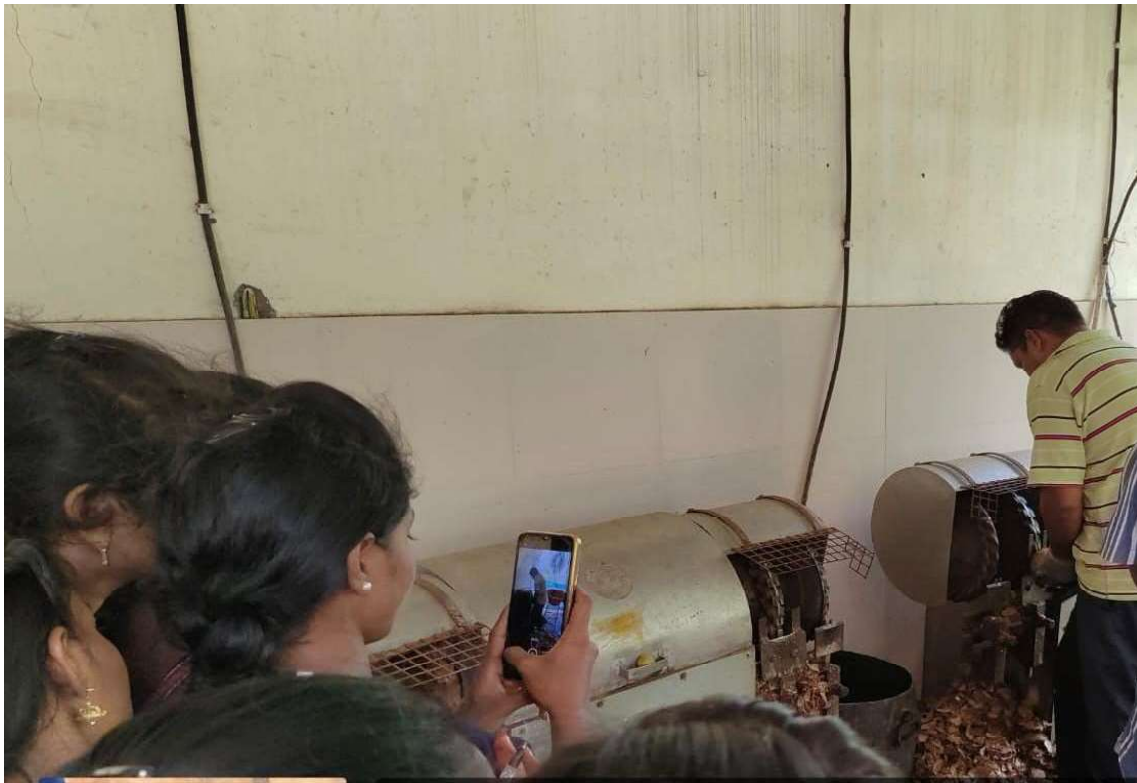
Students are observing the how copra(dried coconut kernels) is chopping into pieces through cutter driven by electric drive.
