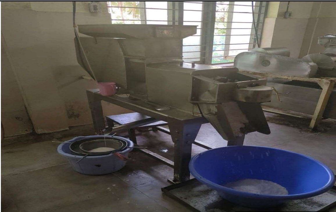
Crushing in expeller: Chopped and roasted copra is crushed in oil expeller in two stages.
